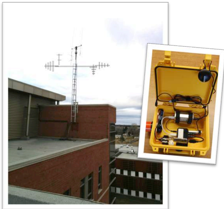
Above Left: projected tower set-up on top of UQAR roof (planned for January 2016) Above Right: The "Sensor Gnome" is the radio-receiver that connects to the antennas and records signals emitted by tagged birds
